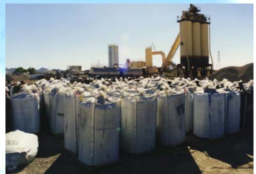
Rubber does not cause smoke at hot-plants, above, a hot plant during production of A-R. near Tucson, AZ.
