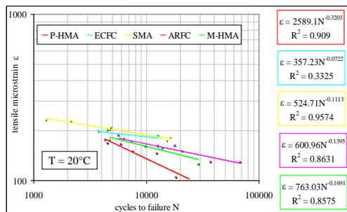
Failure = the number of cycles to the flex point of the permanent deformation evolution law
