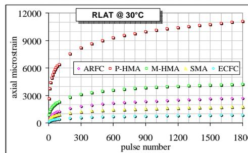
RLAT results are presented as mean values of two identical tests for each material studied
