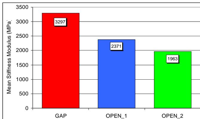
**Figure 11.** Indirect Tensile Stiffness Modulus of several AR mixtures @ 20°C
