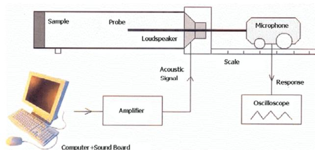
**Figure 17.** *Sound absorption test setup*
