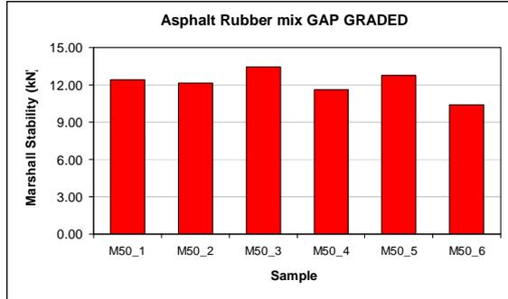
Figure 4. Marshall Stability of a Gap Graded AR mix
