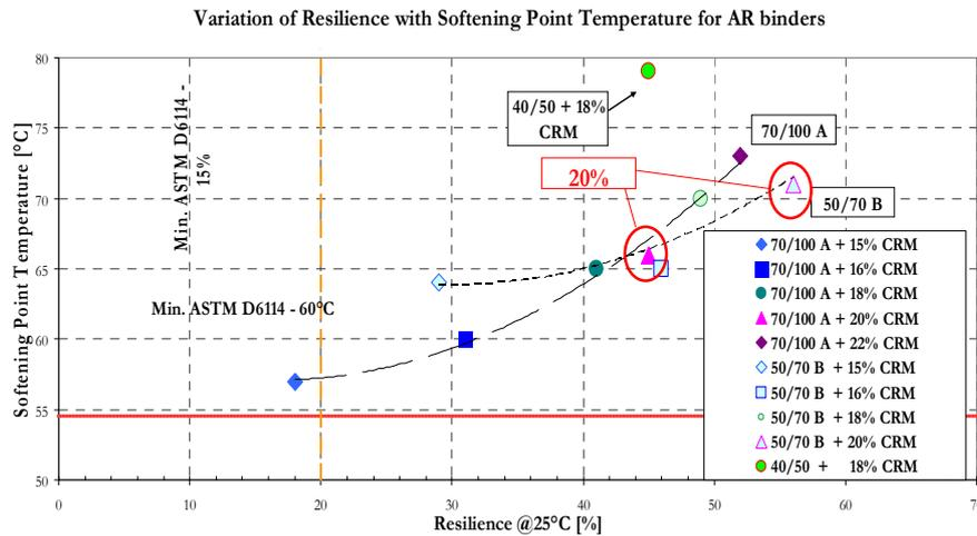
**Figure 2.** Variation of resilience with softening point for Asphalt Rubber with different percentage of CRM
