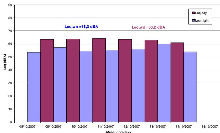
**Figure 15.** *In situ* noise measurements (one week)
