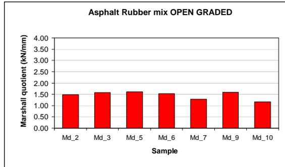
**Figure 9.** Marshall Quotient of an Open Graded AR mix
