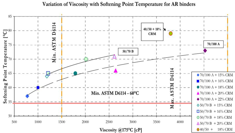
**Figure 1.** Variation of viscosity with the softening point for Asphalt Rubber with different percentage of CRM
