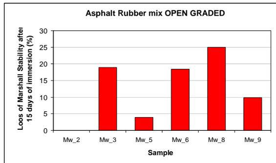
**Figure 10.** Loss of Marshall Stability of an Open Graded AR mix
