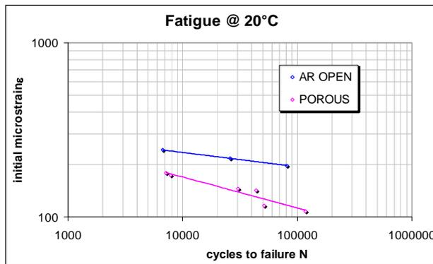
**Figure 12.** Fatigue behavior of an ARFC Open Graded AR mixture
