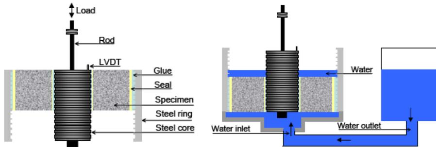
**Figure 20.** CAST setup for dry test (left) and wet test (right)
