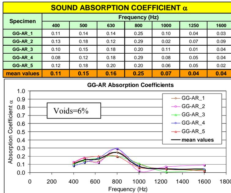
Figure 19. Absorption coefficients of Gap Graded AR mix
