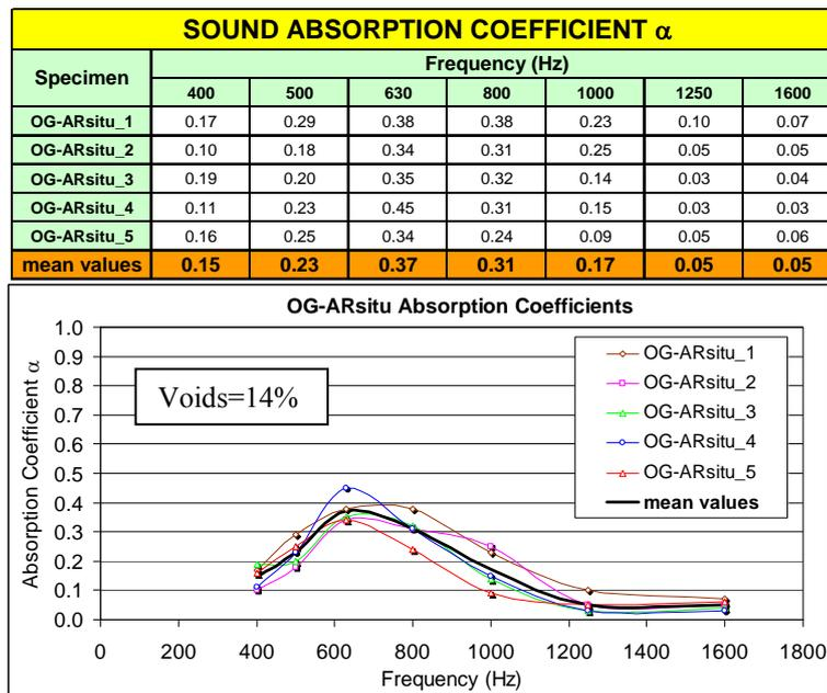
**Figure 18.** Absorption coefficients of Open Graded AR mix
