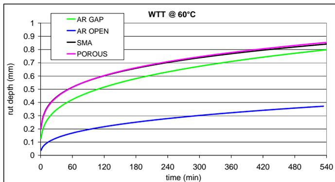
**Figure 13.** Rutting behavior of AR mixtures
