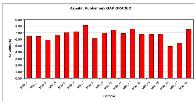
**Figure 3.** Volumetric properties of a Gap Graded AR mix
