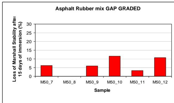
Figure 6. Loss of Marshall Stability of a Gap Graded AR mix
