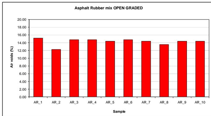
**Figure 7.** Volumetric properties of an Open Graded AR mix
