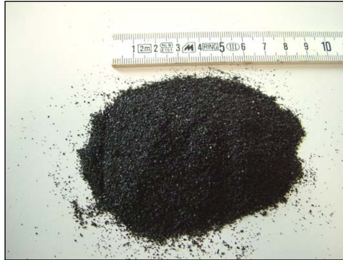
Figure 1. Crumb rubber used for binder modification
