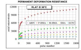
RLAT results are presented as mean values of two identical tests for each material studied
