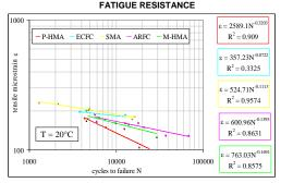
Failure = the number of cycles to the flex point of the permanent deformation evolution law
