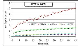
ARFC performance is comparable with that of SMA and ECFC showing virtually no deformation
